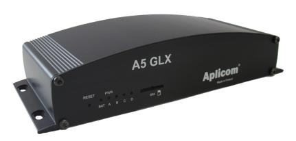
APLICOM A5 GLX is designed for professional applications where for example driver performance information and engine data is utilised with FMS CAN, GPS and GLONASS tracking, driver identification and accurate mileage information. Power management, internal and external events handling, and optimised data communications are also supported features. Voice call interface offers an effective and safe way of communication between the office and the driver.
