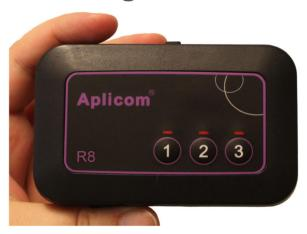
R8 IS A PORTABLE, READY TO USE, TRACKING UNIT suitable for all kinds of mobile tracking applications. The buttons on the device provide easy status or alarm messaging and the inbuilt, large, 25mm patch antenna guarantees a good GPS reception. Positioning can be activated based on time interval, motion or pressing one of the buttons.
