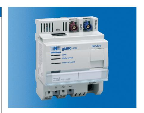
The gMUC-GPRS controller from Dr. Neuhaus Telekommunikation GmbH enables multi-line wireless remote data reading from domestic and industrial supply meters by means of GSM/GPRS network or DSL connections. Measurement values for electricity, gas, water and heat are automatically transmitted to one or more centrals locations using common Internet standards.
