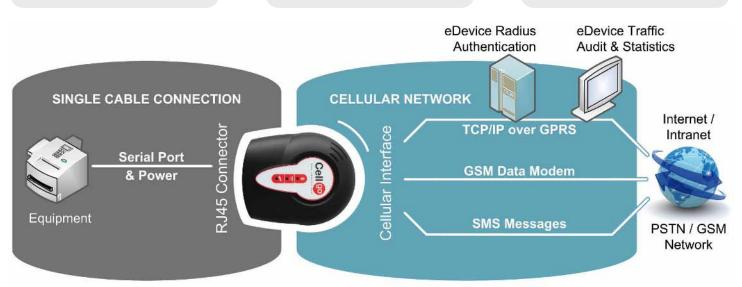
Cellgo, by virtue of its low-cost achieved through hardware and software optimization, is the easiest way to enable electronic equipment to communicate wirelessly. The existing serial port is simply connected to the RJ45 connector on the Cellgo, allowing Internet connectivity through cellular networks using standard AT and AT# commands.
