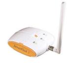
This miniature device is equipped with a 2.4 GHz IEEE 802.15.4 compliant radio, a 32bit MIPS CPU, and an on-chip AES cryptographic unit for hardware-acceleration.
