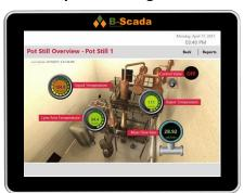
Customer uses Status Device Cloud to monitor distillery equipment in this IoT pilot project. The project allows customer to monitor temperatures and flow rates in real time, and remotely control valves when needed.
