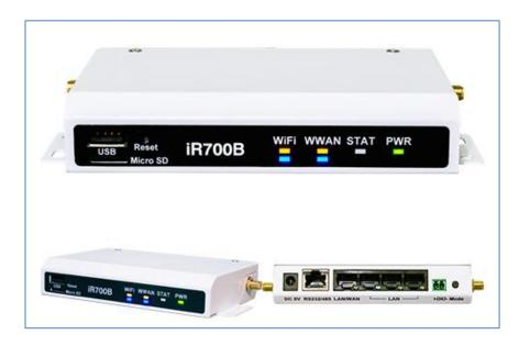
As an LTE-enabled wireless router, it is being used in solar power farms, metered parking, digital signage, and video surveillance, among others.
